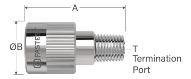
Actuation: Manual Twist Pressure Rating: 275.6bar (4000psi) Vacuum Rating: Vacuum Leak Rate Capability: 1E-5cc/sHe Connection / Application Method: Manual Grip Method: Continuous Thread Dim A: 52.07mm (2.05in)
